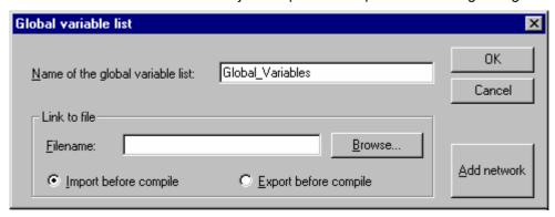
Click on the button **Add Network** to get the options for defining the network properties of the current variables list. If you have set up several network connections, then you can configure several connections for each Global variable list.
