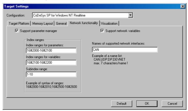
Activate the option **Support parameter manager** in the dialog 'Target Settings', tab 'Network functionality'. Enter the **Index ranges for parameters** and **variables** (parameter lists of type 'Parameter' resp. 'Variables') and the **Subindex range**.
